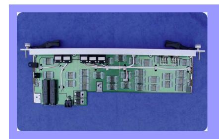
The RTM Thermal *Blade* is used in conjunction with the Thermal *Blade*. A RTM connector connects the two boards, with power being supplied by the Thermal *Blade*.
